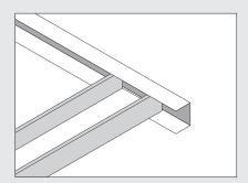
1: Mark the horizontal ceiling at the required height on all adjoining walls. Mark the lower side of the U-profile and fix it to the wall using 6-mm dowels in predrilled holes. Determine and mark the anchor points for the C60 profiles. Always install the first adjustable suspension bracket max. 300 mm from the wall. Distribute the remaining adjustable suspension brackets with a max. spacing of 1200 mm
