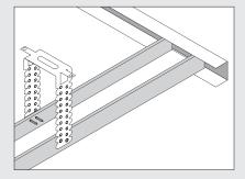
2: Hold a main profile with the opening facing upwards and screw on the adjustable suspension bracket to the side of the profile at the desired height. Bend back any excess section of the adjustable suspension bracket. Assemble the main profiles longitudinally using C-connectors, and terminate the main profiles in the U-profile.
