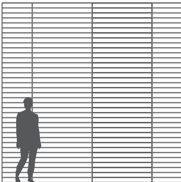
Troldtekt v-line 2way 6 installed in horizontal stack bond.
